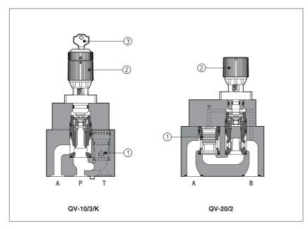
QV are flow control valves with pressure compensator ① (the controlled flow rate is indipendent of pressure variations), designed to operate in oil hydraulic systems.
